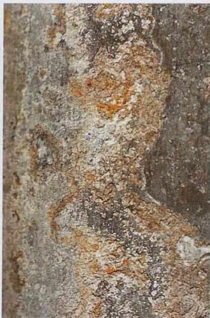
Fig. 4: A large area of wet storage stain clearly showing local corrosion of the base steel.
