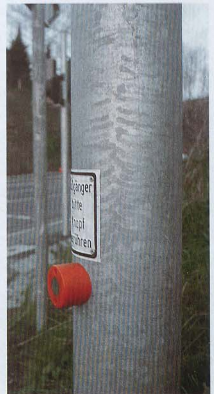
Fig. 2: A minimal amount of wet storage stain seen on a signal mast. This is not significant for the galvanized coating. However, it must be removed before any duplex coatings are applied.
