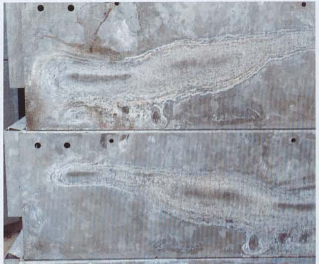
Fig. 1: A hot dip galvanized water container after storage for several months outside. The tightly packed conditions prevented sufficient circulation of air, resulting in the formation of wet storage stain.
