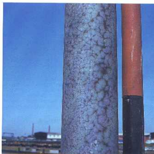
Figure 4: Grey reticular appearance of the zinc coating.
