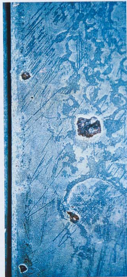
Fig. 3: Cathodic protection on damaged surface areas of a zinc coating
