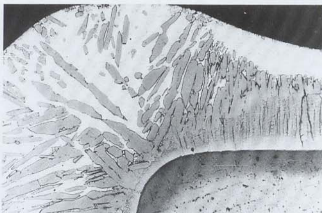
Fig. 6: Zinc coating on a component edge (micro-edge).
