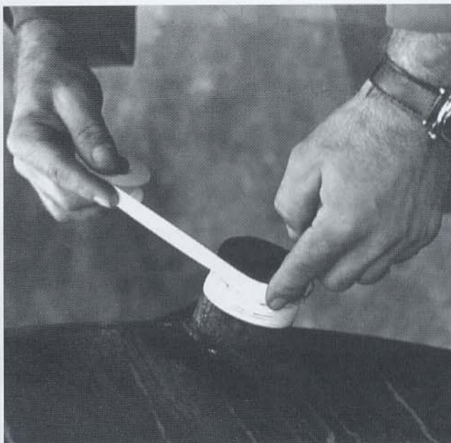
Fig. 1a: Wrapping threaded bolts with a cloth based tape will protect them from being zinc coated.
