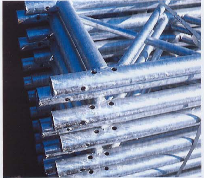
Fig. 1: A zinc lump on hot dip galvanized tubular structure
