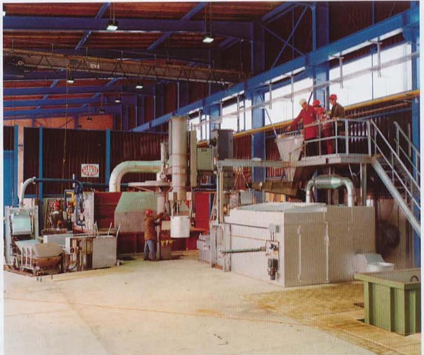
Fig. 1 : An automatic hot dip galvanizing plant for small components.
