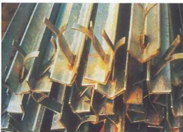
Figure 2: Flaws in the galvanized coating due to weld slag not being removed.
