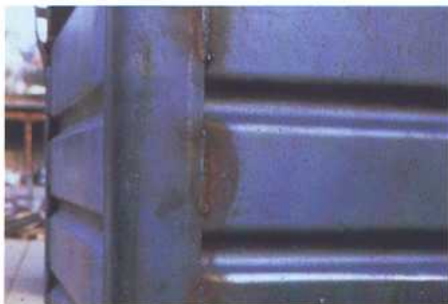
Figure 1: Residue etched into the area around the weld seam of a greased container (in this instance before galvanizing) may create problems.
